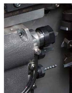
By simultaneous 3-path control system, diverse simultaneous processing such as ID processing, OD processing and back processing is possible. High productivity can be achieved.
