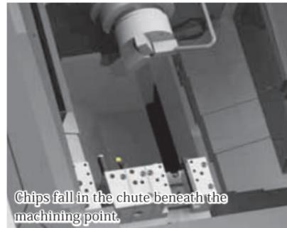
Chips fall in the chute beneath the machining point.
